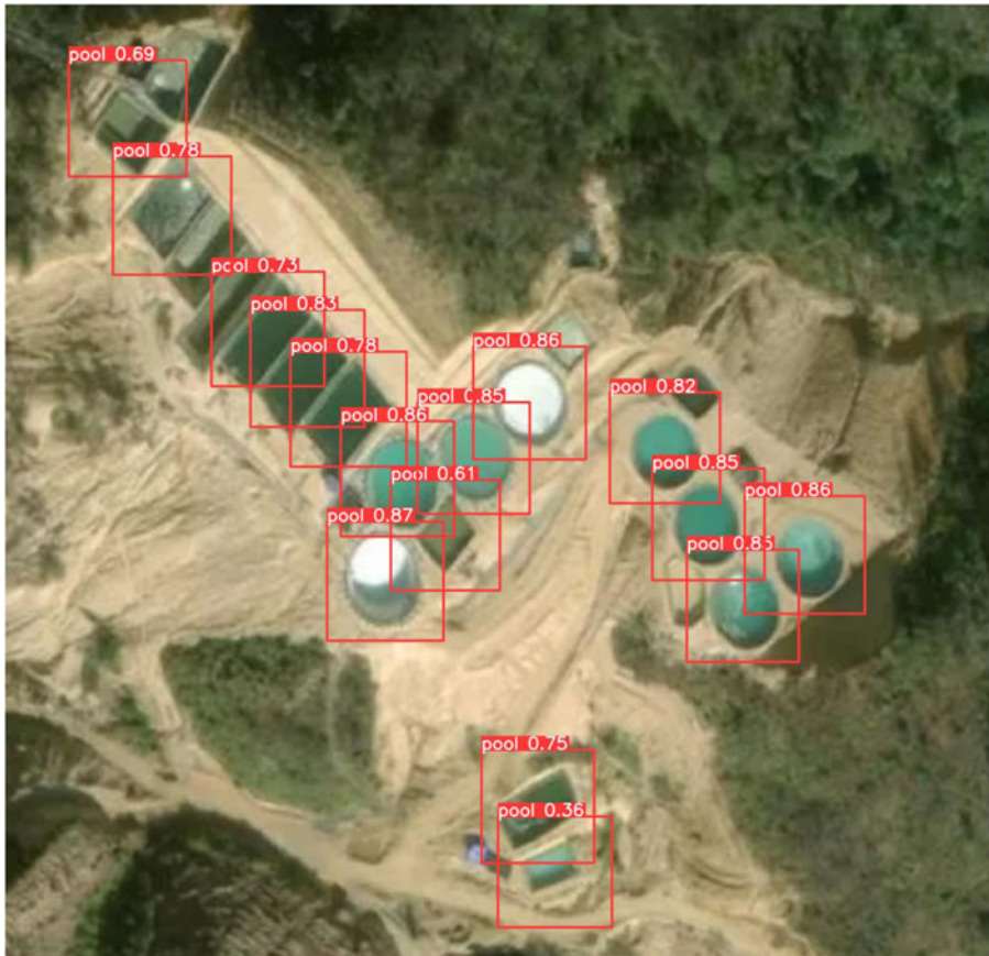
Figure 4. Computer vision model trained to identify rare-earth mining pools. Source: Authors' analysis of Mapbox Basemap imagery.
